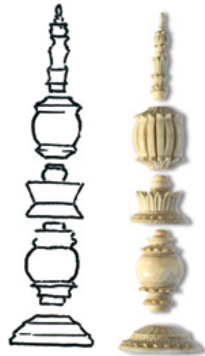
Fig. 2: Turned chessman prior to carving. / 8043
