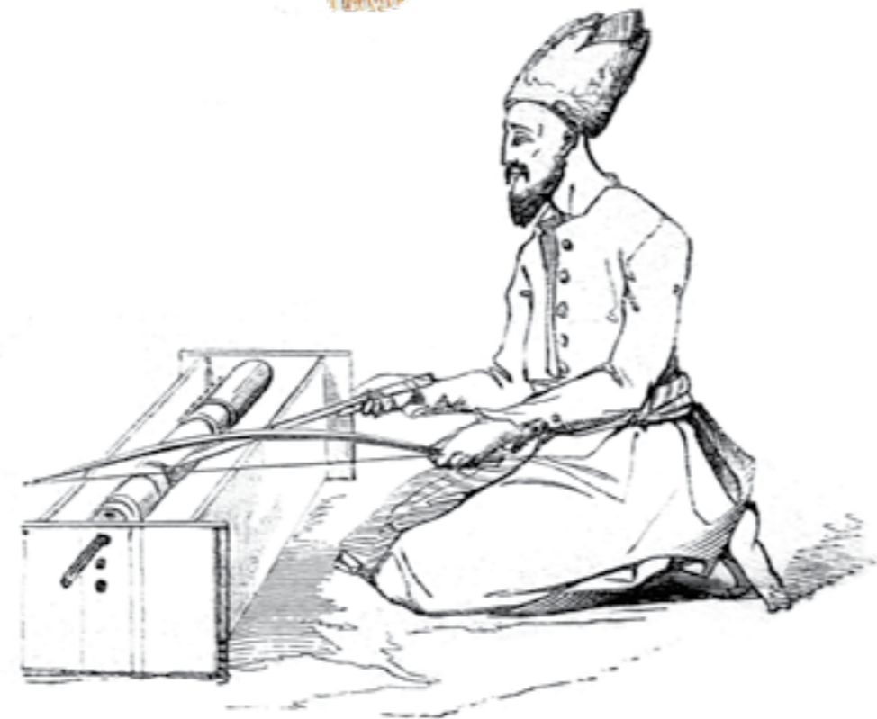
Fig. 5: Bow-driven lathe (Persian lathe), after John Jacob Holtzapffel, Turning and Mechanical Manipulation , vol. IV, London 1881, p. 7 Fig. 6. / 8046
