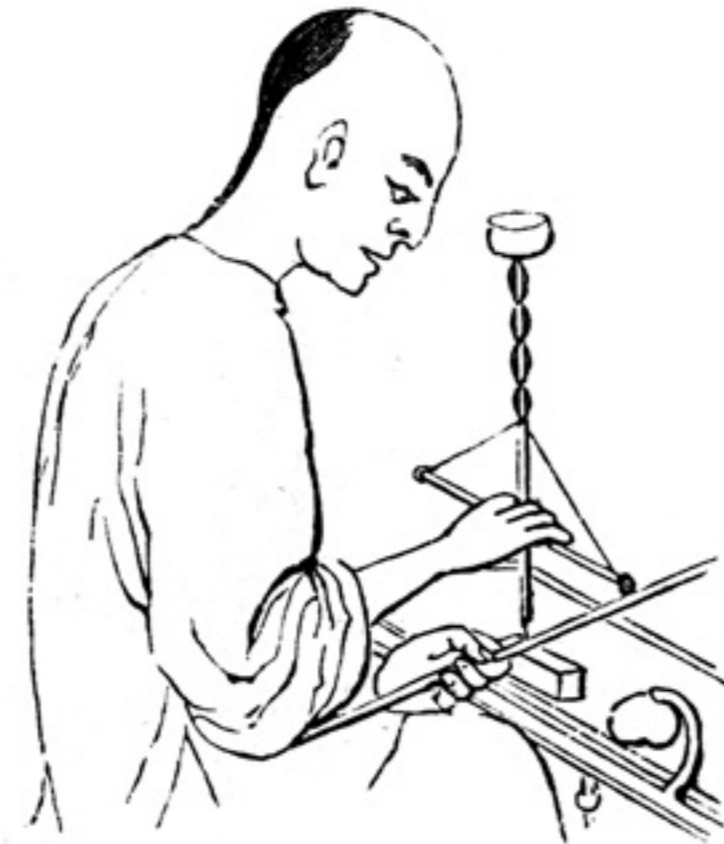
Fig. 9: Bow-driven drill, after John Jacob Holtzapffel, Turning and Mechanical Manipulation , vol. IV, London 1881, p.4, Fig.3. / 8050
